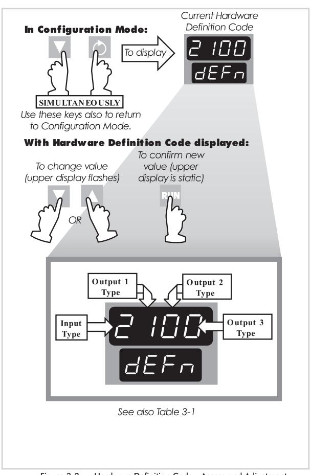
Figure 3-2 Hardware Definition Code - Access and Adjustment
